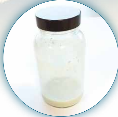
Mixing of ferrous sulphate and potassium ammonium phosphite produces a heavy precipitate of iron phosphites
